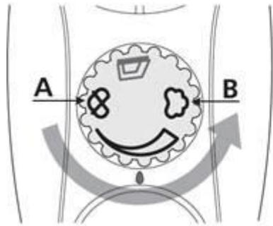
The amount of steam produced is regulated by the Steam/Dry switch.
