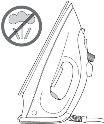
3. The steam will stop once the iron is placed in the vertical position.
