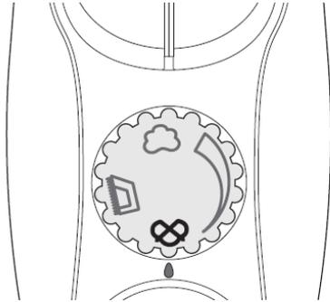
To iron without steam, rotate the Steam/Dry Switch to the dry setting ∞.
